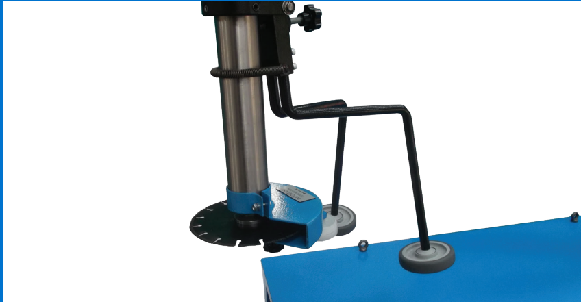
Stator Cut Off machine for removal of old windings prior to the burn off operation.
