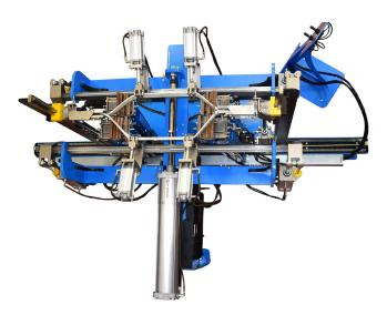
Radius forming in small coils presents some challenges but Rotary have developed a compact, robust radius forming solution for smaller loops. Mounted on the swivel bar, the radius forming system can be positioned close to the slot holders.
