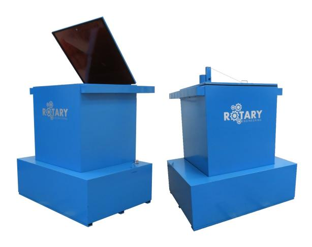
Rotary Varnish Tanks comprise a two tank system, one tank is a dip tank whilst the other tank is for storage when the varnish is not in use. This keeps the varnish in good condition. The top dip tank is used to soak the windings and is suitable for a wide range of propriety vanishes including trickle and water based types.
