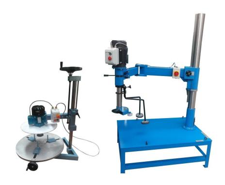
SC2 Bench mounted stator cut off machine for stators up to 460mm high
