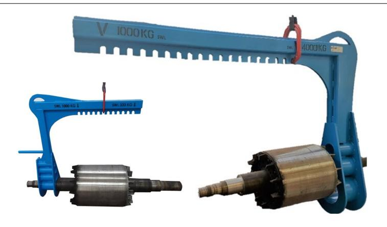
The rotor lifter is a heavy duty lifting device for handling large rotors up to 4,000kg in weight. It is designed to balance the rotor by means of a slotted support for the shaft and an adjustable masterlink. This equipment is invaluable for lifting rotors in the horizontal plane. Slots are provided in 3 / 4 difference sizes to suit different shaft diameters
