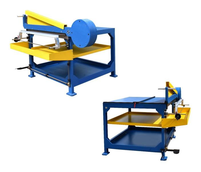
Heavy duty insulation cutter with guides to ensure insulations are cut perfectly straight.
