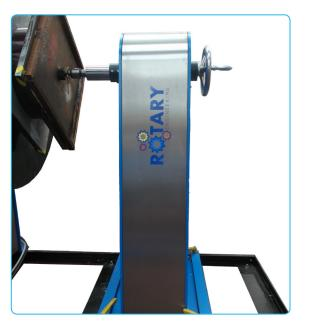
Tailstock on adjustable rails, used to
