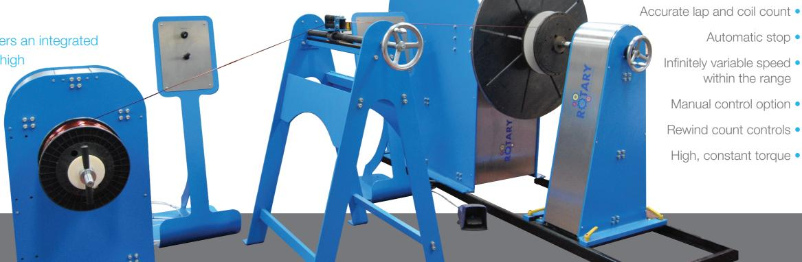
Pneumatic braking system gives adjustable control of wire tension. Face plates and formers are available.
