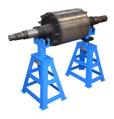
Rotary armature stands are used to support an armature during the repair process. Armature stands are sold in pairs, one with a fixed height and one is height adjustable by means of a handwheel. This set up allows the engineer to set the armature level where shaft diameters on each end of the armature are different.
